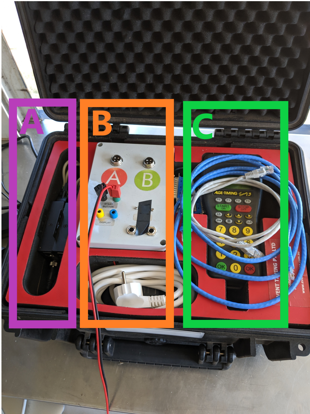
In this image, A are the Moxa nPort servers. B is the interface between the Timy and the displays / buttons. C is the timing device, an Alge Timy3, itself.
